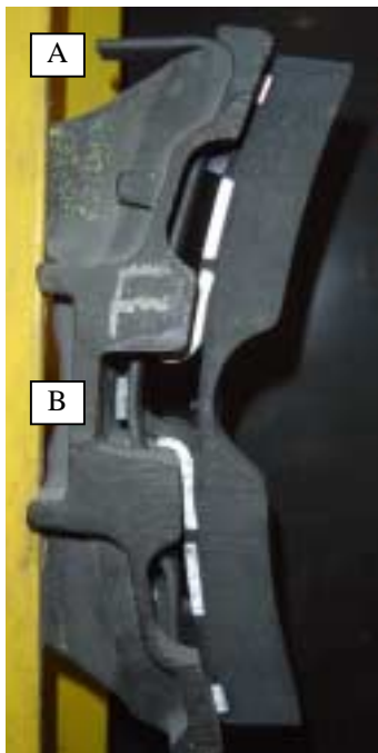
Figure 1 - X-section of brake shoe installed on brake head with a properly inserted Key.
