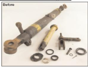
Reconditioned SA's receive new stainless steel ball bearings and races, all alloy over-travel tubes, cone nut housings, composite seal inserts, conical springs, seals, retaining rings, control rods, sleeve nuts and lock nuts. Steel cone nuts are replaced with new brass nuts. Springs, rod weldment, housings, and castings are inspected to strict standards and reused or replaced with new.
