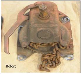
All reconditioned HB's receive *upgraded* new front housing assemblies with sealed main shaft bearings. Movable cams and back plate bushings are 100 % replaced with new. All 9300, 9300-3 and 7500 hand brakes built prior to 1993 must have new winding drums applied. All remaining components are inspected to strict standards and replaced with new if necessary.
