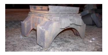
The Shear Pads continue to deliver nearly twice the wheel life of conventional adapters.
