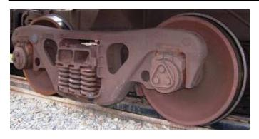
This S-2-E Truck with Split Wedges and Shear Pads has been in service for over **700,000 miles** on a high side coal gondola.
