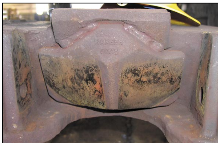
Bolster pocket is in excellent condition with normal wear patterns
