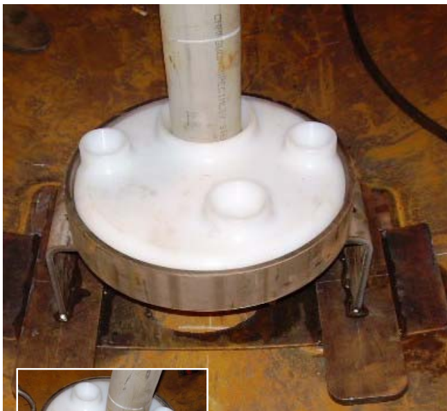
AFTER: Example of the Eduction Pipe Assembly equipped with the ZefTuf® Eduction Pipe Guide prototype.
